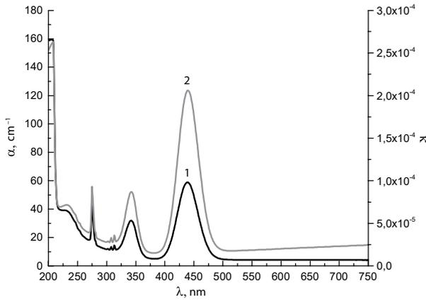
**Figure 3.** Spectral functions of absorption coefficient and extinction coefficient: (1) absorption coefficient and (2) extinction coefficient
