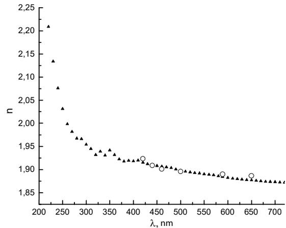
**Figure 5.** Dispersion functions of refractive index obtained using (o) Brewster method and (▲) reflection at low incidence angle close to normal
