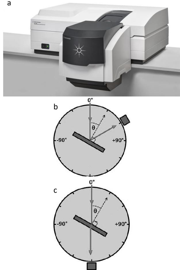
**Figure 1.** (a) Appearance of the Cary 5000 spectrophotometer with a UMA accessory, (b) specular reflectance measurement experimental setup and (c) transmittance measurement experimental setup.
