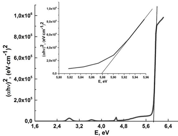
**Figure 4.**  $\text{Gd}_3\text{Al}_2\text{Ga}_3\text{O}_{12} : \text{Ce}$  optical band gap determination using Tauc method
