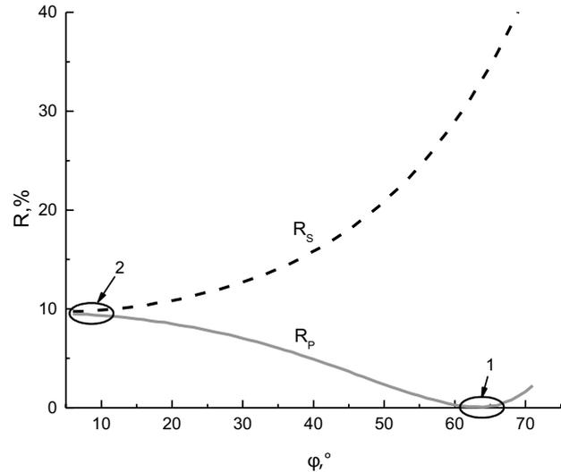
**Figure 2.** Reflection angular spectra for  $p$ - and  $s$ -polarized light: Region 1 for Brewster measurement of  $n$ ; Region 2 for measurement at low light incidence angle close to the normal
